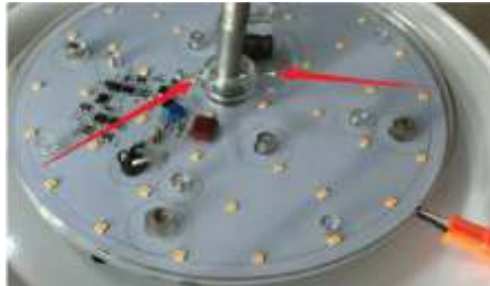
Tighten the Screw as shown above to mount on Centre Rod
